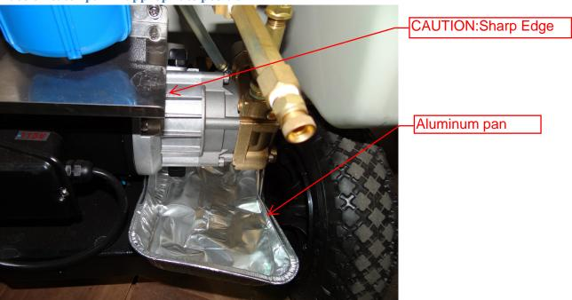
Unscrew fill cap, recommend using 20mm wrench.
