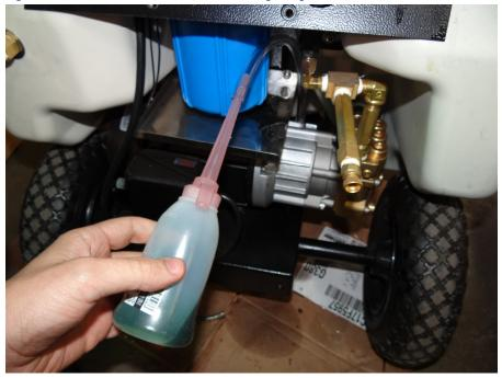
After the pump is full of new oil, reattach the fill cap.
