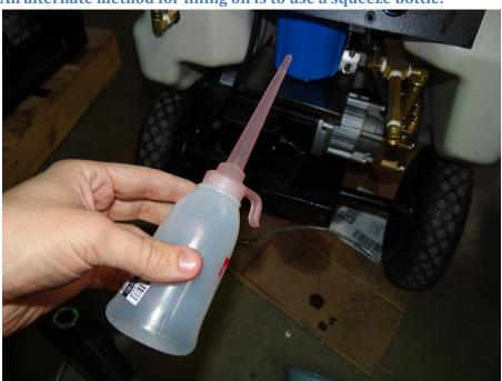
Squeeze oil from container into the pump until it is full.
