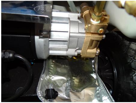
Remove oil pan, and attach drain plug.
