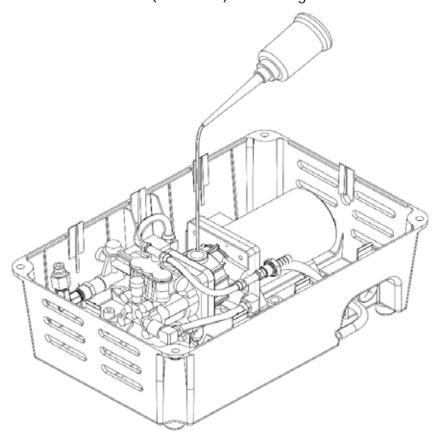
7.2.11 Tighten the oil fill plug. Wipe up any spilled oil. Visually check the pump and motor to ensure all bolts, screws and connectors are tight and in good condition.
