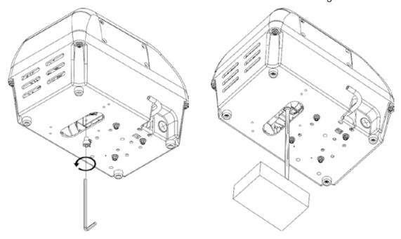
7.2.7 After the oil has drained, reinstall and tighten the drain plug.
