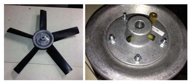
Step 4: Put the new fan blade assembly onto the fan motor shaft with the hex screws facing the fan motor housing. The fan motor shaft has a flat on it. One black hex screw must line up with the flat. Front of fan blade assembly must be flush with end of fan motor shaft. Align fan motor assembly and firmly tighten the hex screws ensuring one hex screw seats on the flat surface of the fan motor shaft.
