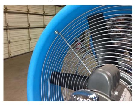
Step 2: A 5/32" long T-Handle Hex Key or a 5/32" socket Hex tool with extension is needed to access the black hex screws, near the shaft, on the fan blade assembly.
