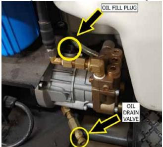
Figure 4 – Oil fill plug and drain valve location.
