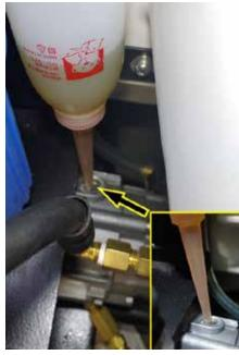
Figure 8 - Vertical bottle orientation.
