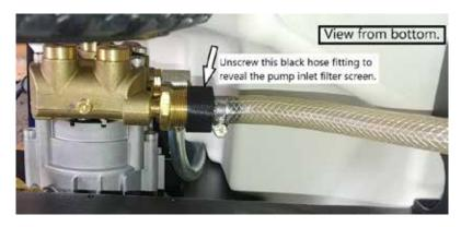
Figure 10 – Location of pump filter screen.
