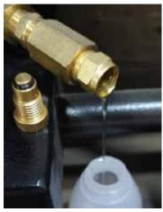
Figure 5 - Oil drain valve with end cap removed.
