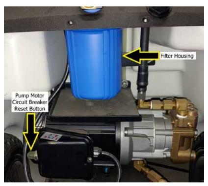
Figure 9 – Location of filter housing and circuit breaker reset button.
