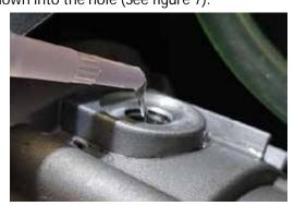
Figure 7 - Horizontal bottle spout filling the pump with oil.
